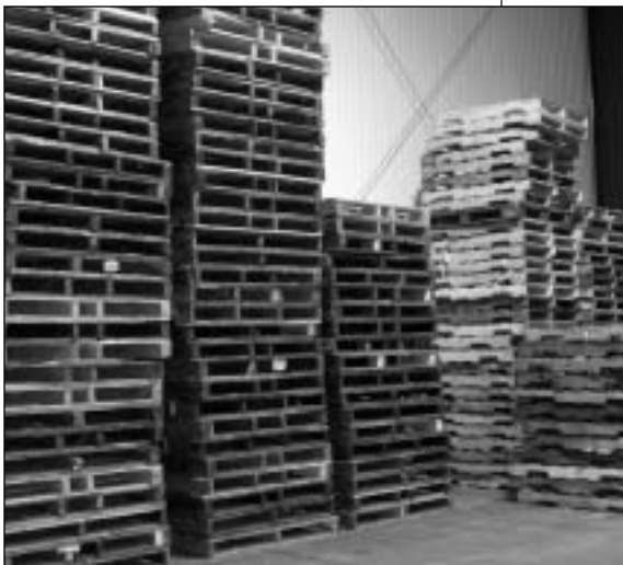
Photo shows storage of wooden pallets. Due to fire safety regulations, pallets can be stored to maximum of 20 units high.
