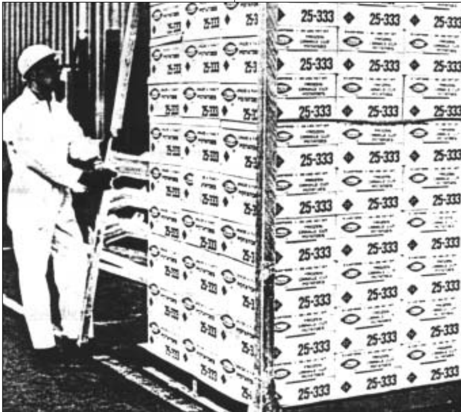
With the addition of corner angle stacking aids for protection against crushing, Simplot can stack double cube loads two high in storage.
