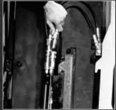
2. Connect quick-change hydraulic couplers
