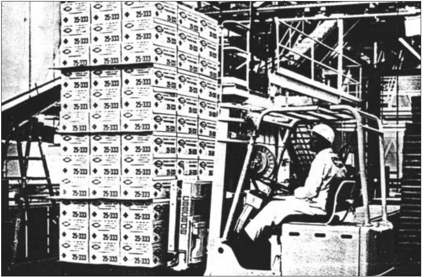
J.R. Simplot Company automatically palletizes double cube loads of 108 cases for frozen storage. Cascade's Load Push/Pull hauls them away from the palletizing center.
