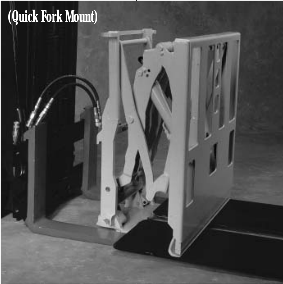
2. Connect quick-change hydraulic couplers
