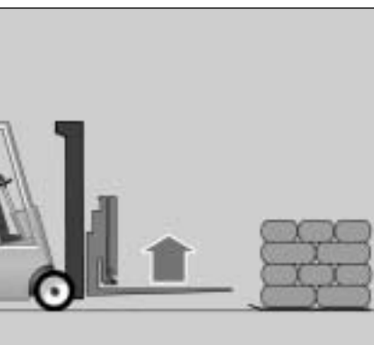
2. Raise the platens about three inches above the floor
