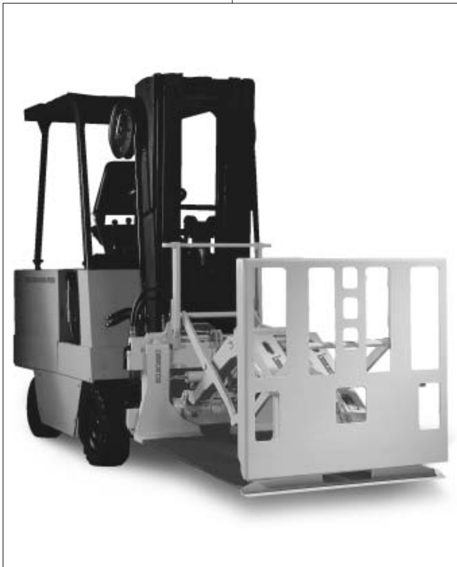
Figure 1: Slipsheet palletless handling system
