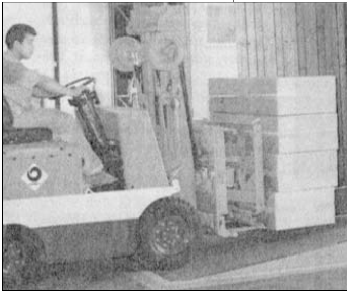
A lift-truck with a push/pull attachment loads an ISO container with electrical appliances. Slipsheet shipping is increasing in Japan due to a new law banning highway vehicle overloading.
