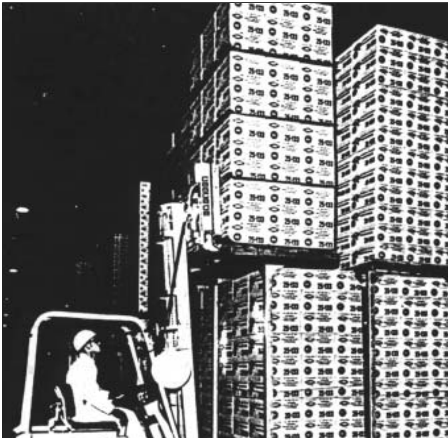
Cascade's Load Push/Pull stacks double cubes two high in frozen storage.
